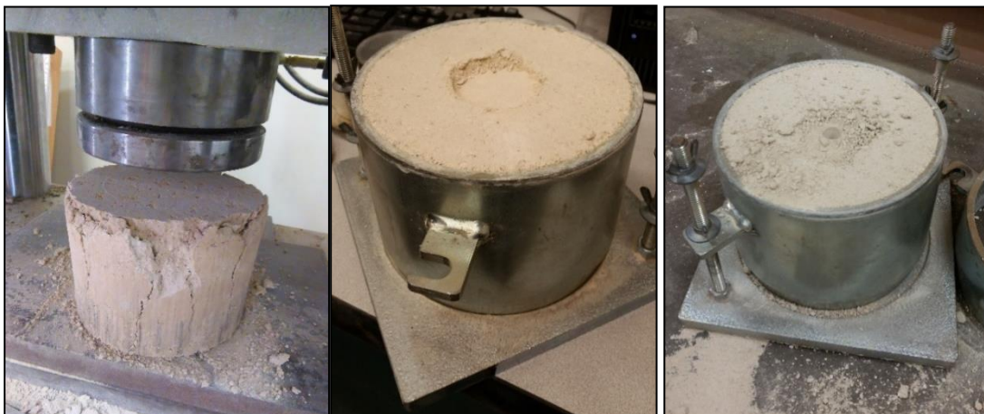
Figure 9. Specimens after (a) UC, (b) CBR, and (c) penetrometer tests
