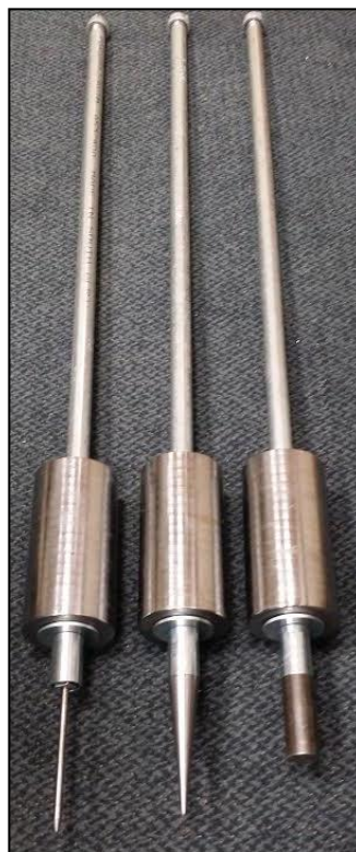
Figure 1. Penetrometers with a nail, cone, and cylinder extensions
