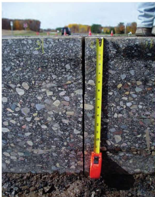
Different Asphalt Mixtures in the Pavement Structure
