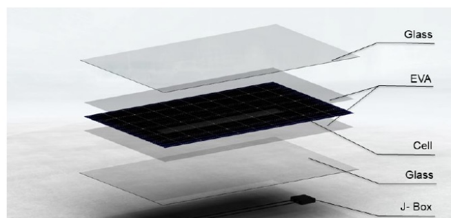
Figure 9. Dual glass module structure (layers)
