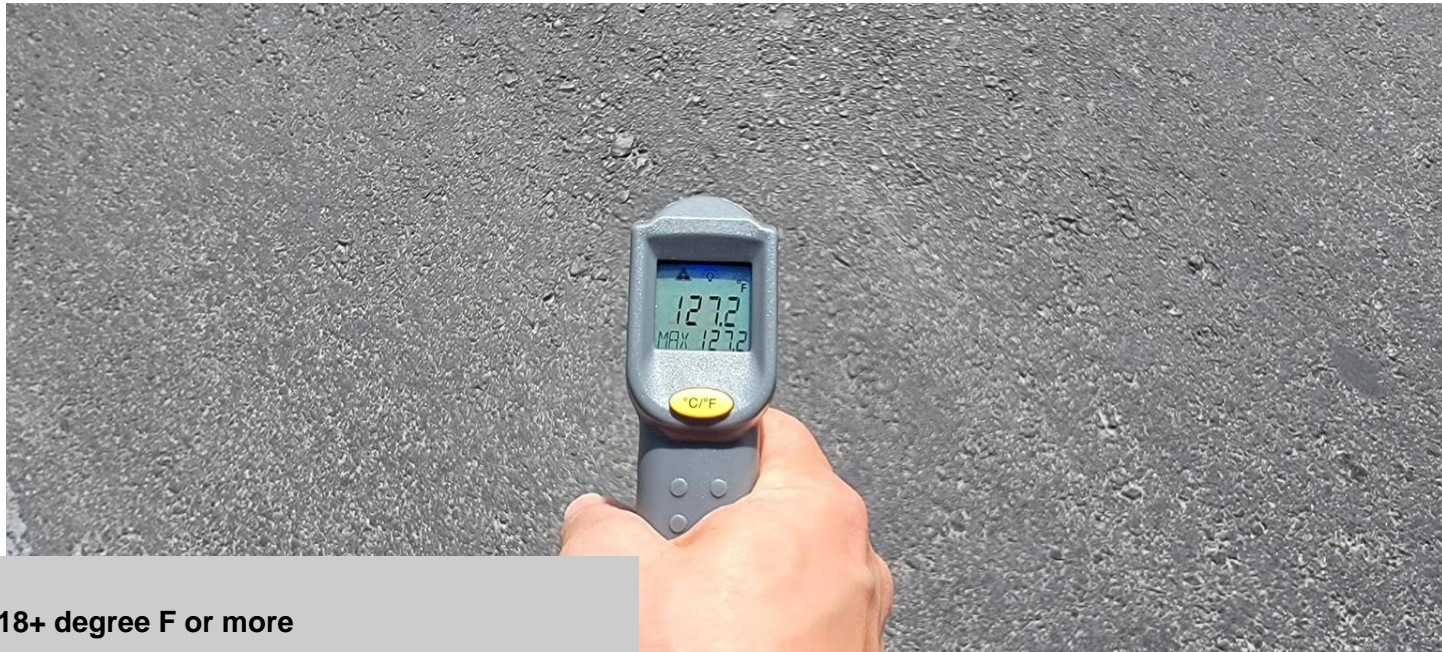
Asphalt Surface @ 127.2 degrees F
